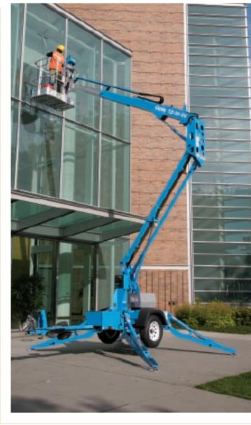
Though rugged and heavy-duty, the TZ<sup>™</sup>-34/20 is lightweight enough to use on lawns, slate or gymnasium floors. Simply put, it meets the challenges of just about any working environment.
